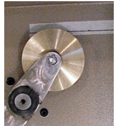
Fine Wire assembly aligned to marked wire path. Shown with right - to-left wire direction.
